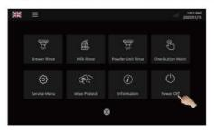
Step 3: The screen pop-up prompts. Are you "power off", click "OK" machine turns to power off mode, click "Back" to cancel this operation, the screen is off but light is still on(press the screen more than 3 seconds to wake up the machine)
