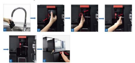
√ The mixer unit has been removed and cleaned.
